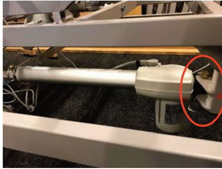
Depending on which direction you want the chair/bed to rotate and then rise to aid the transfer between sitting and standing, the rotate and tilt actuators can be moved to the opposite side of the frame which will make the chair/bed rotate the other way. The chair/bed will rotate through 90° toward the opposite side of the frame where the actuators are mounted.
