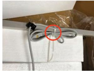
Once the cables are free from the ties they can be inserted into the actuator in the bed end. To do this you will first need to remove the securing clip as shown in the image below left.
