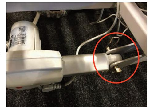
The rotating function actuator is also only attached to the bed frame at one end so the other end needs connecting to the bed frame. This is again done by removing the pin and swinging the actuator round to the bracket (shown in the red oval in the image to the right) and then inserting the pin before locking it in place with the loop. The electrical cable connecting it to the control box is already connected.
