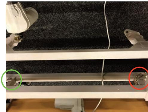
The image on the left shows the tilt locking pin at the head of the bed in its standard position, shown by the red circle. Note that in the standard position it is on the opposite side of the bed frame to the actuator.
