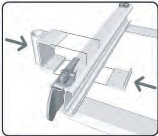
Attach the bridge support bracket to the bridge by sliding the 'U' shaped bracket over the bridge so that height adjustment tube connector is on the outside of the bridge.
