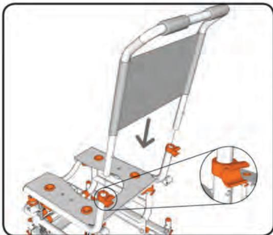
Insert the back rest frame into the seat base.
