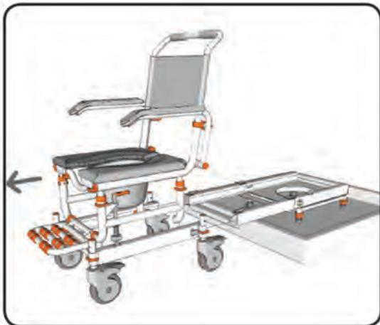
Ensure the primary brake securely locks your Showerbuddy in position on the wheeled base before disconnecting the bridge.
