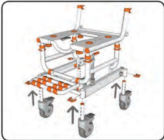
Insert each 5" castor wheel into the wheeled track.
