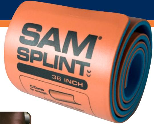
The **SAM® SPLINT** is based on an ancient construction principle: curves are strong. The **SAM® SPLINT** is built from a thin core of aluminum alloy, sandwiched between two layers of closed-cell foam. The splint is exceptionally pliable. Bent into any of three simple curves, it becomes extremely strong and supportive for any fractured or injured limb.
