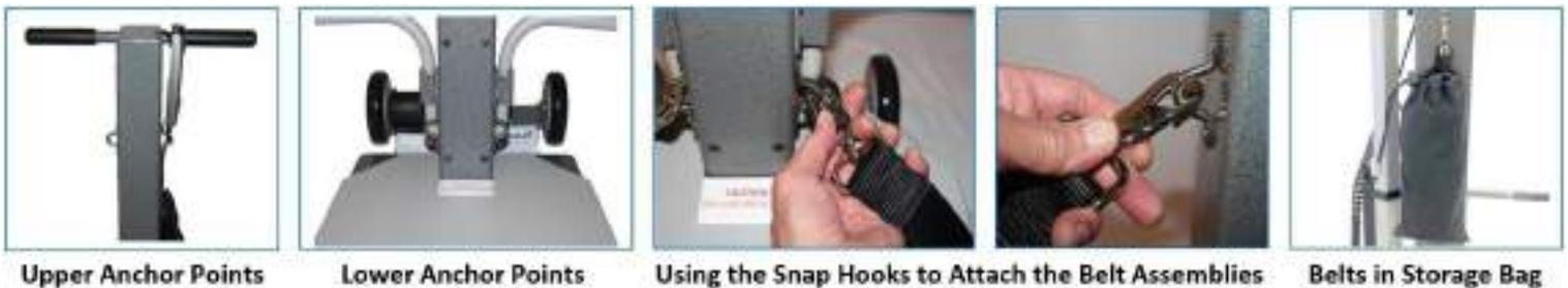
NOTE: Depending on the circumstances, you may choose to use the waist belt only. The anchor points and belt assemblies also allow for additional configurations, (such as crossing the chest of the person being lifted by attaching one belt assembly to the upper left and lower right anchor points and the second belt assembly to the upper right and lower left anchor points).
