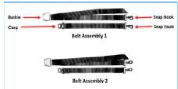
In use, they are secured to the HFL's upper and lower belt anchor points, (located on the HFL's main column), using snap hooks at the end of each belt assembly. The upper belt assembly and anchor points can be used as a chest belt and the lower belt assembly and anchor points can be used as a waist belt. When not in use, they are rolled-up and placed in the column-mounted storage bag.
