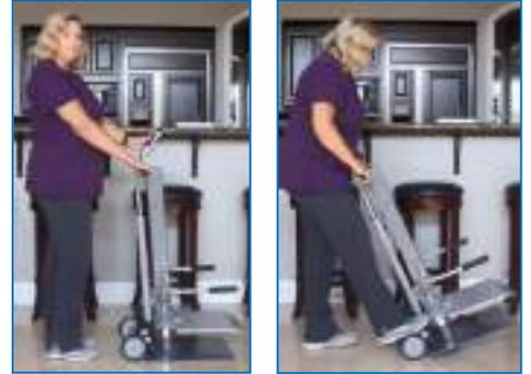
1. Stand behind the HFL and place one foot on the back of the unit. Then gently tilt the HFL backwards by pulling the handle towards you. You can now pull or push to HFL to the fallen person.
