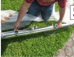
Removal of the screws to fasten the C-tube
