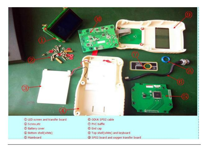
**MD300A Parts Price** 1 transfer board \$181 2 Screw,etc \$10 3 Battery cover \$3 4 Bottom shell(white) \$31 5 Mainboard \$77 6+7+8 ODU6 SPO2 cable, PVC baffle, End cap \$26 9 Top shell(white) and keyboard \$52 10 SPO2 board and oxygen transfer board \$72
