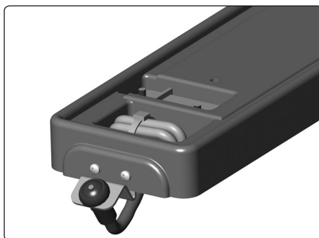
Fit the control button cabling and connection contact with the cable ties in the armrest.
