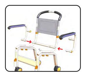
Fit Left Hand Arm (part #500-043) and Right Hand Arm (part #500-045) by positioning the axle (smaller diameter) part of the tube against the hollow tube across the rear of the Seat Frame (part #500-021) and sliding into this tube.
