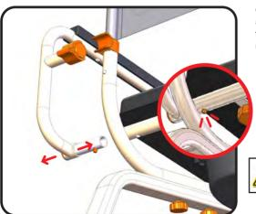
depress the push pin (part #500-269) fully allowing the arm rest to be pulled outwards from the seat frame tube. To re-fit the arm. reverse this action.
