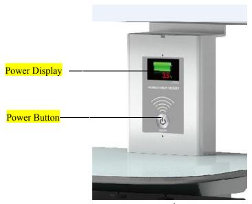
Turn on the control panel power button "O", then turn on the computer power and monitor power.
