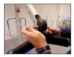
Withdraw the security pin and the outer sleeve bush, then remove the spreader bar.
