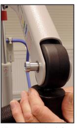
Align the nylon bush / 'Cam-shell' mouldings with the boom crosshole and insert the outer sleeve supplied with the kit (0YJH0090).
