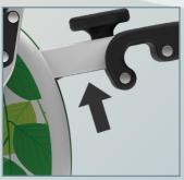
The battery is located in the bottom of the carrying handle. It can be changed by tightening the knob fully (Clockwise) and flipping the battery case, which is held in place by a magnet, out of the carrying handle.
