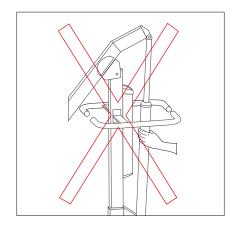
Do not place the Pool lift on an sloping surface.
